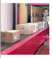
Specially designed weigh modules for conveyors in warehouses and airport logistic centers absorb strong lateral shocks from moving parcels, palettes and containers. Terminals with dedicated software for in-motion weighing process correct weight results.
