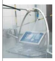
METTLER TOLEDO operates several ISO/IEC 17025 : 2005 accredited test labs, which perform tests according to internationally applicable EN/IEC standards. Static and dynamic loading as well as all kinds of environmental effects such as shocks, vibrations, temperature, water and dust impacts can be simulated.
