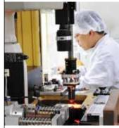
Robots affix strain gauges to the metal body inside a clean room. All METTLER TOLEDO factories are equipped with advanced production technologies and apply state-of-the-art methods for production management. They are certified according to ISO9000 and ISO14000.
