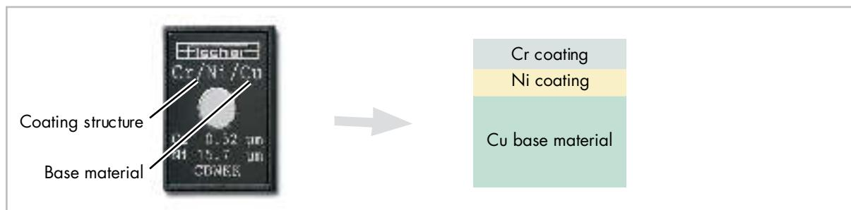
The identification of the calibration standards contains the information, whether a coating thickness and/or a concentration can be calibrated: **d** = coating thickness, **c** = concentration, examples:
