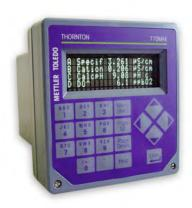
The 770MAX is Thornton's most advanced instrument for on-line measurement. It offers six-channel multiparameter measurement capability for resistivity/conductivity, TOC, pH, ORP, dissolved oxygen, ozone and temperature plus flow, pressure and level. The configuration flexibility of the 770MAX is unmatched, allowing up to 16 measurements from the 6 input channels with unique features such as specialized temperature compensation modes and derived measurements.
