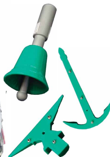
Detail of the finished, fettled castings
