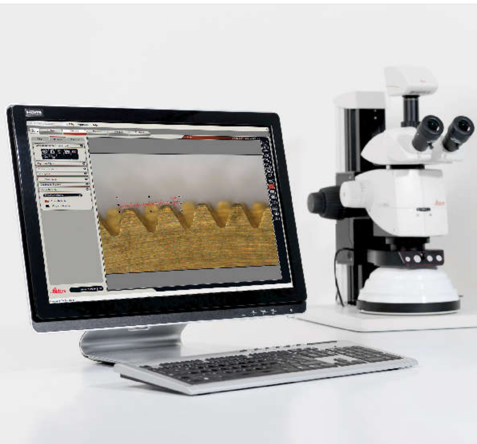
Reticule to estimate component symmetry and diameter.
