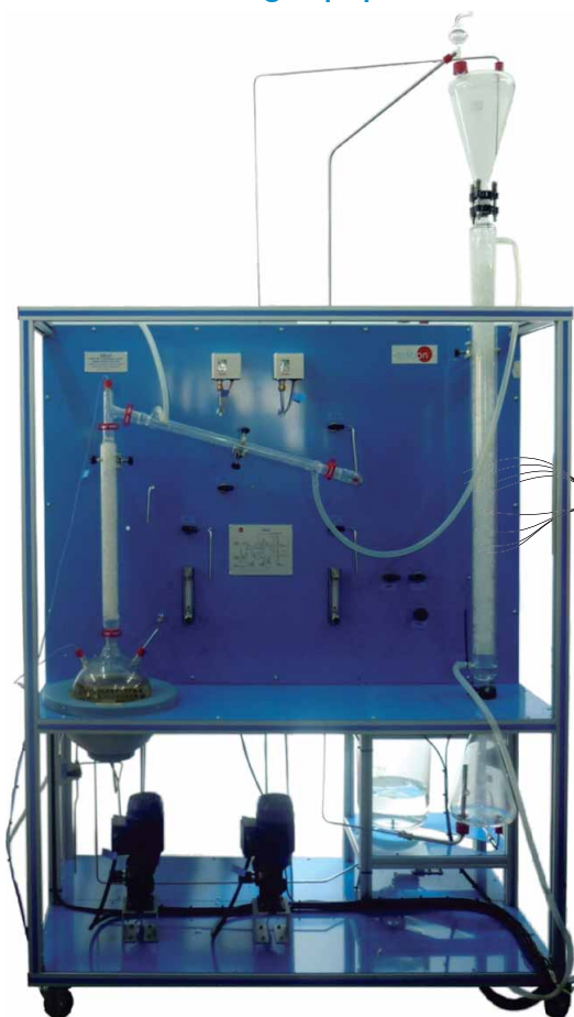
① Unit: UELLC. Liquid-Liquid Extraction Unit
