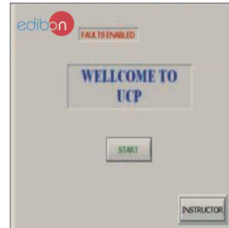
(1) Welcome screen. From the instruction button (with instructor's password) the faults mode is activated.
