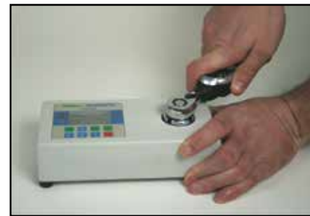
TT Shown Testing Torque Wrench
