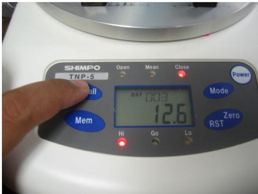
Example from the picture above shows 3 data is saved (003) and the last value is 12.6. Pressing the Zero/RST button, the last data is eliminated (CLr will appear on the screen). Pressing the Zero/RST button again deletes the next data stored in the TNP torque meter.
