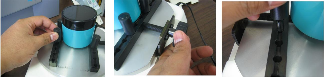
It is important to make sure that all the jigs are flush to the moving brackets. Each one of these jigs has set pins which slides into place inside the grooved brackets.
