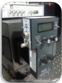
• PDS-1, PMT detector
