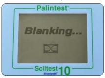
The Soiltest 10 Bluetooth will determine the absorbance due to the sample colour at all wavelengths simultaneously and store in temporary memory for use in analysis.
