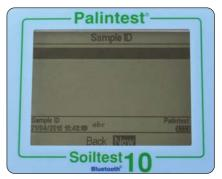
To create a new Sample ID, select Sample ID and use the up/down keys to select a blank field. Select New and press OK.
