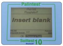
Insert the Blank cuvette and press OK.
