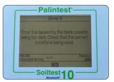
Ensure the blank cuvette is being used, not the sample plus reagent cuvette. Sample colour can be reduced by dilution with clean water; the dilution selected should take account of the expected concentration of parameter under test.
