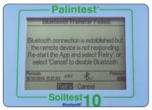
The Soiltest 10 Bluetooth is not receiving a response from the Palintest Aqua Pal app but the remote device is connected. This will appear 10s after a result transmission has started and no valid response has been received.
