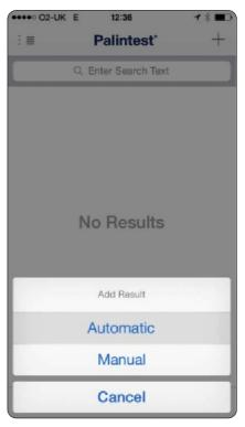
To connect the Soiltest 10 Bluetooth press the '+' symbol in the top right hand corner of the device screen. This will produce the list of all locally advertising Bluetooth SMART devices.
