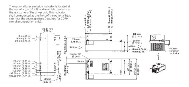
Sapphire Driver Unit Operate, Control and Monitor Sapphire Laser Heads
