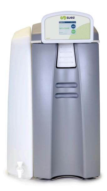
The Select Analyst is a compact unit ideal for laboratory use, delivering a steady supply of >  $1M\Omega$ .cm pure water for laboratory tasks using carbon pre-treatment, reverse osmosis and deionisation.
