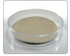
**NutriDisks** are the option most commonly used with the Wagtech Test kits. **NutriDisks** are larger than the standard aluminium petri dishes supplied in the kit but are still designed to fit into the standard petri dish rack. This allows up to 7 **NutriDisks** to be incubated at the same time.
