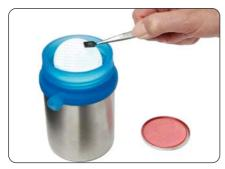
20 Starting at the far edge of the petri dish, use a rolling motion to place the membrane filter on top of the absorbent pad. This will prevent air being trapped between the pad and membrane filter.
