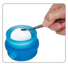
**6** Lock the membrane filter in place by pushing the filter funnel firmly into position in the blue rubber base. Take care to not touch the internal surface of the filter funnel with your hand.
