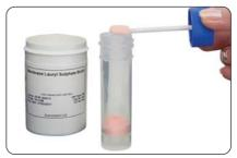
8 Fill the MMD with sterilised water to the lower lip and screw the lid on tightly.
