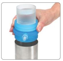
**NOTE:** If the sample is not to be collected in the sampling cup part of the membrane filtration unit, then the filter funnel/base assembly can be inserted into position in the sampling cup straight away.
