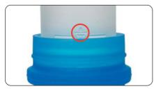
**8** Pour the water sample into the filter funnel up to the 100ml graduation (or less if using a smaller sample).
