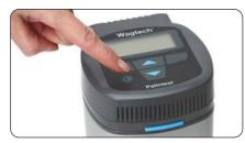
A red LED in the right hand corner of the incubator lid indicates that power is supplied and the incubator is on. The backlight will illuminate automatically on key press.
