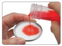
18 Ensure the pad is well saturated with a small excess of MLSB visible at the edges. This should equate to between 2.5 and 3.0mls. If too much media is dispensed, simply pour the excess away. Place the petri dish back down on the work surface.
