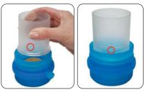
Once the flame has virtually extinguished, invert the filter funnel and silicone rubber base components of the MFU and insert into sampling cup as shown below.
