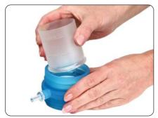
7 Ensure the filter funnel is aligned correctly in the 'Filtration' position, indicated by the graphic on the side of the filter funnel.
