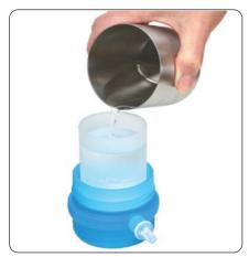
**9** Discard the excess water from the sampling cup then insert the filter funnel/base assembly into position in the sampling cup. Care is needed to prevent sample spillage from the filter funnel when assembling.
