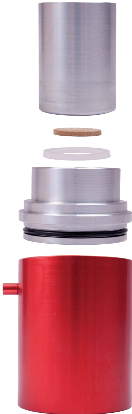
The assembly of the reservoir tube filtration base
