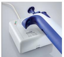
Scan your pipette LabX uses the RFID reader to access the pipette's data. Once scanned, LabX displays the pipette's complete profile, including its serial number, manufacture and calibration due date, and any unique attributes assigned.
