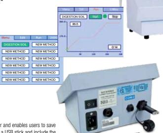
The USB port is conveniently located at the back of the controller and enables users to save detailed reports for laboratory audits. The reports are saved onto a USB stick and include the following data: date and time of the sample run, instrument serial number, temperature log in 15 second intervals and safety messages. The controller is perfect for quality control, research and method development.
