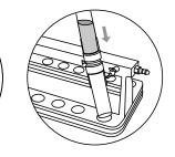
Flip the tube-filter assembly over so that the tube containing the sample is now on top. Attach the assembly to the manifold, inserting the valve into the filter port.
