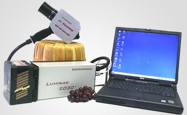
Luminar 5030 "Le Vigneron" handheld Analyzer for grape and liquid wine measurements
