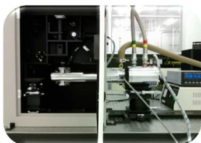
Cryostat system For 2 inch wafer sample
