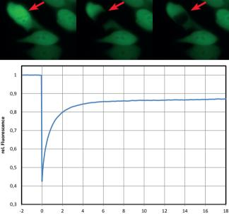
Fluorescence intensity over time curve for a photobleaching experiment. The LAS X software automatically calculates the recovery curves for your experiments.
