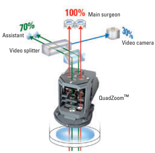
Leica Microscope featuring QuadZoom™ The main surgeon benefits from 100% light, even if a video camera is added.
