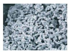
A Promet": Typical structure of a metal powder (Ag) created by in ert gas condensation (nan opowder). This antimicrobial nanosil ver coating reduces in fect ious agents on the instrument and their transmission tousers.
