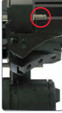
Installed too high
