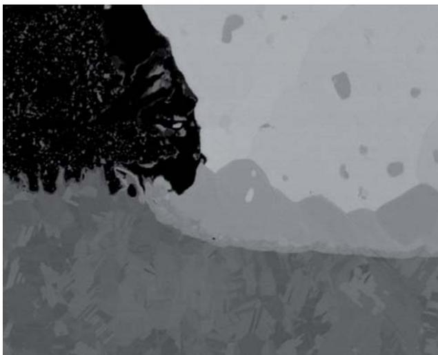
Solder ball after ion beam polishing
