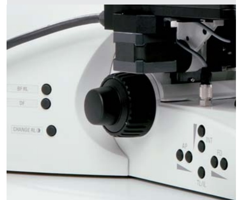
Configure specific illumination and diaphragm settings with the buttons on the left front side.
