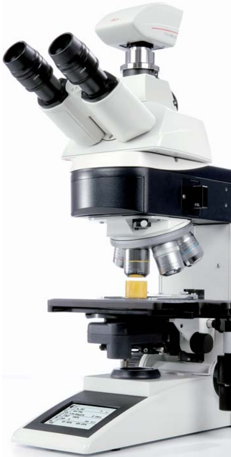
Leica DM4000 M LED with incident light and transmitted light axis
