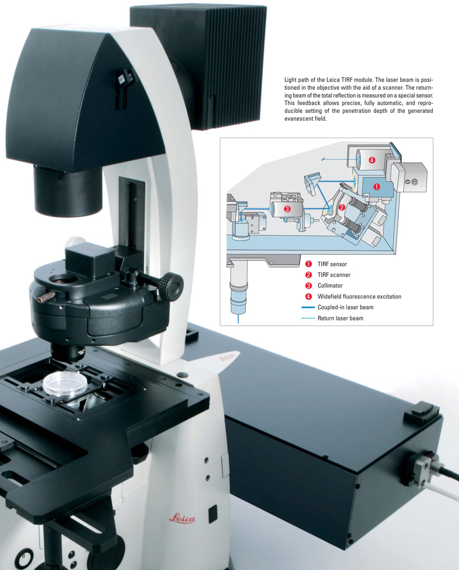
Light path of the Leica TIRF module. The laser beam is positioned in the objective with the aid of a scanner. The returning beam of the total reflection is measured on a special sensor. This feedback allows precise, fully automatic, and reproducible setting of the penetration depth of the generated evanescent field.
