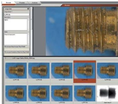
**LAS Archive Basic** ① – Microscope and camera data can be stored with the image and combined with user defined text fields for display on a data form. This data is freely searchable and additional files and audio recordings can be attached to the image.
