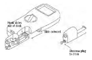
NOTE: O2 reading will be invalid if the Water Trap Plug is not in place.
