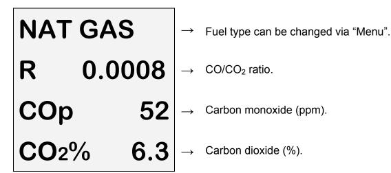
Press send / to print a full combustion test, (or send to PC via optional Wireless module).
