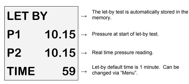
If the let-by test fails simply move the rotary switch to any position other than "tightness" to abort the test.
