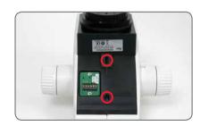
2. Press the optics carrier backwards to the focusing column and screw it in place using your other hand.
