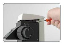
2. Remove the cover of the cable duct.
