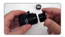
2. Clamp the graticule on the insert, applying moderate pressure. Ensure that the graticule fits tightly.
