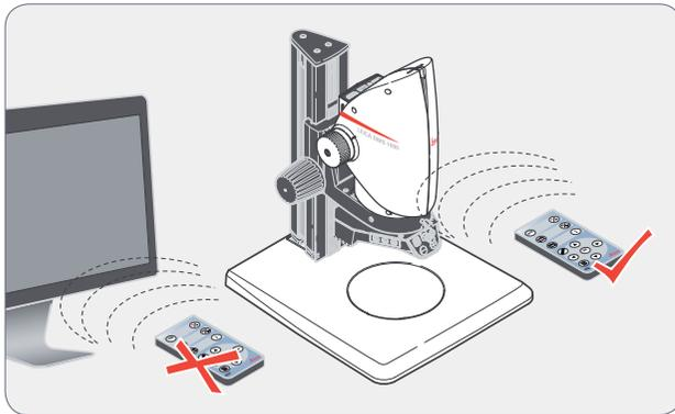
Always keep the remote control for controlling the Leica DMS1000 B pointed towards the microscope's IR receiver.
