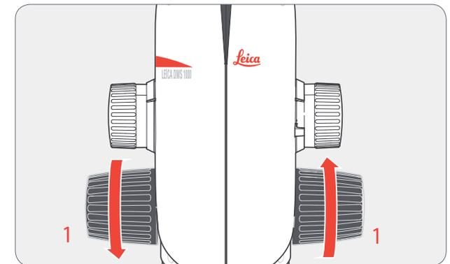
1. Grip the drive knobs with both hands and turn them towards each other until the desired resistance is reached during focusing. On focusing columns with separate coarse and fine adjustment, the outer drive knobs have to be twisted in opposite directions relative to each other.
