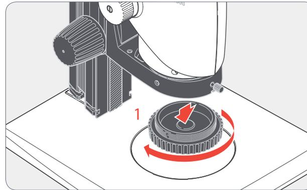
1. Remove the protective cap on the optics carrier by turning it.
