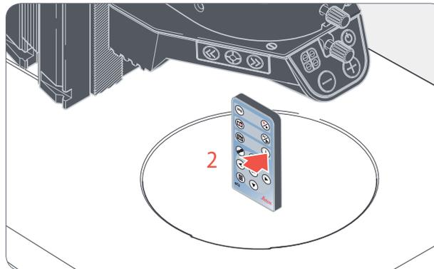
2. Hold the remote control in the beam path so that it faces upwards and press any key.
