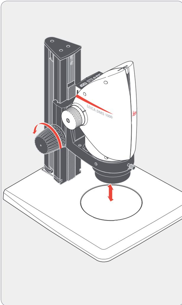
Focusing raises or lowers the microscope using the focusing drive. The specimen detail is brought into sharp focus as soon as it is in the focal point of the objective.
