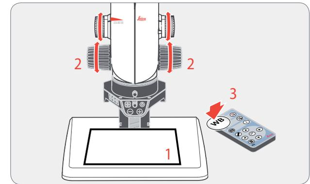
1. Position a gray chart or a gray, neutral object under the microscope so that the entire image field is filled in.
