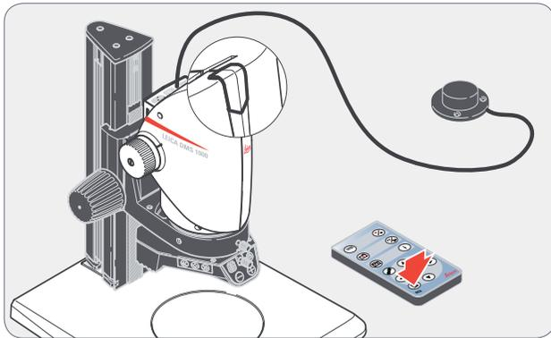
Both the Leica DMS1000 B's front button and optional footswitch can be configured with the remote control as defined by the user.
