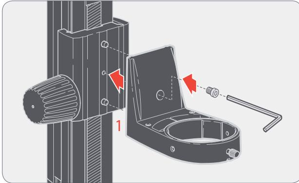
1. Fasten the microscope carrier to the column using the provided Allen key and the screw provided (recommended variant for objectives with a short working distance).
