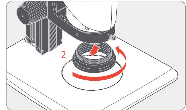
2. Screw the compatible adapter onto the optics carrier.
