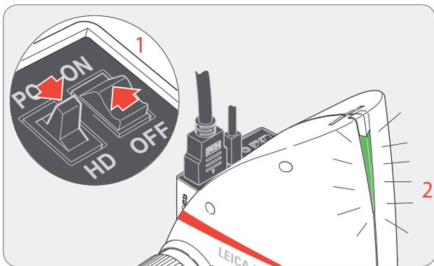
1. Set the on/off switch to "ON" to switch on the Leica DMS1000 B.
