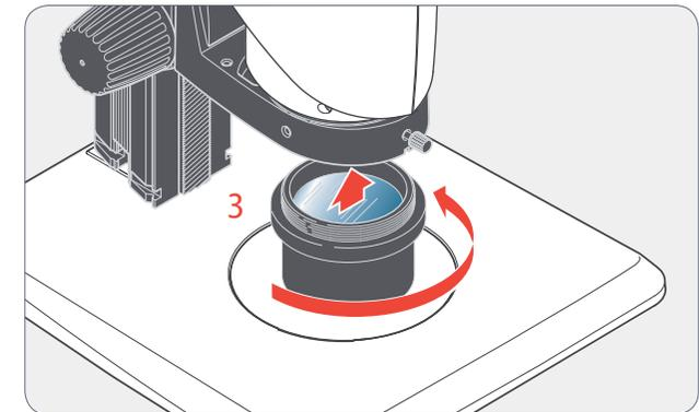
3. Screw the objective onto the adapter.
