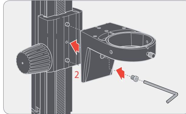
2. Alternatively, the microscope carrier can also be installed upside-down (recommended variant for objectives with a large working distance).
