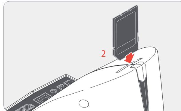
2. Push the SD memory card into the slot on top of the Leica DMS1000 B until it clicks into place.
