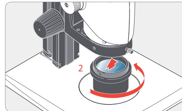
2. Screw the objective into the optics carrier.
