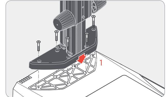
1. Install the column adapter and column to the transmitted light base using the six screws provided.
