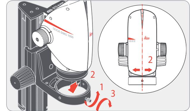
1. Unscrew the clamping screw.
