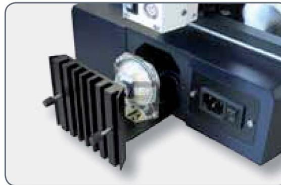
2. Carefully pull out the lamp and mount by pulling them upwards.
