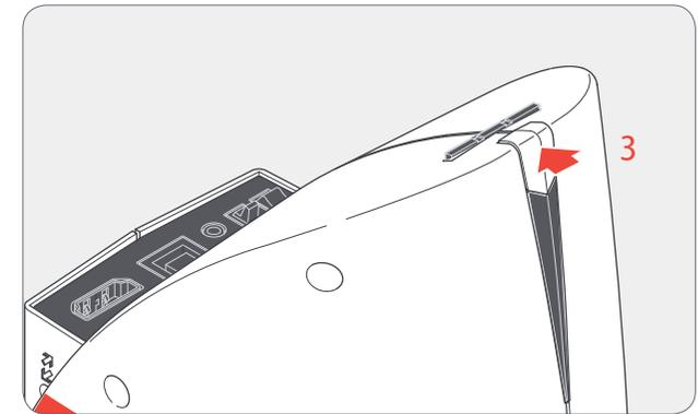
3. Briefly press the Leica DMS1000 B's front button to capture an image.
