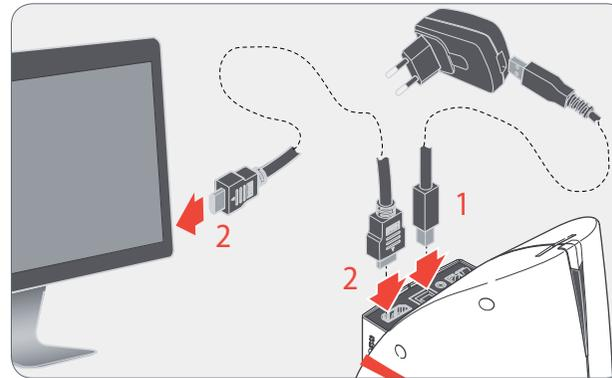
1. Check that the Leica DMS1000 B is properly supplied with power via the USB power supply.
