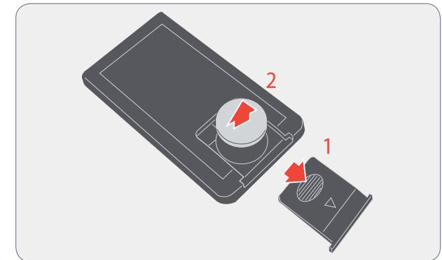
1. Remove the battery cover on the rear side of the remote control.
