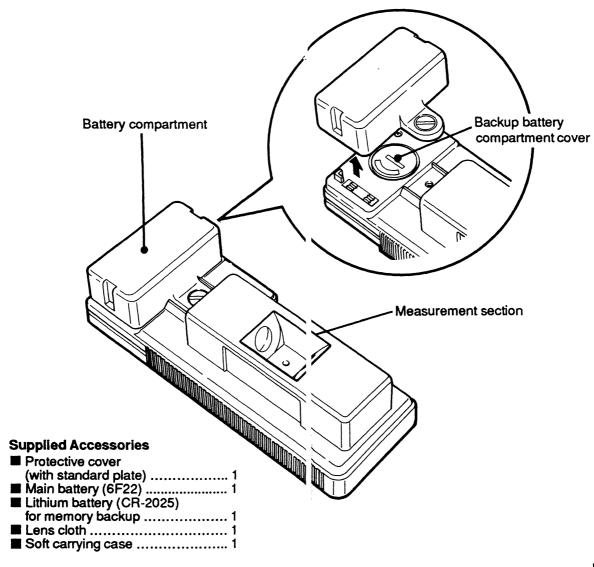
This unit uses two batteries, a 9-V battery for normal operation and a coin-sized lithium battery for data storage and memory backup. When the following display appears, replace the respective battery.
