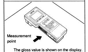
3 When wishing to store the measured data, press the DATA IN button.
