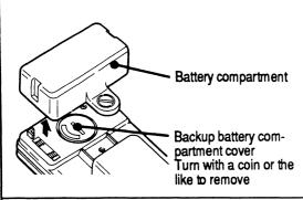
2 Remove the old lithium battery, if inserted.
