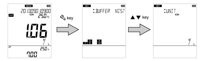
3. Press the ◀ ▶ keys to select the unit and press the ● key.
