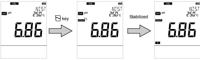
6. Perform the 2nd point calibration. As with the step 2., wash the pH electrode and immerse it in the pH 4 standard solution. As with the step 4., immerse at least 3 cm from the tip of the pH electrode.
