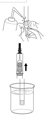
5. Check that the pH value is stable while the pH electrode is immersed in the standard solution, then press the  $\bigcirc$  key.
