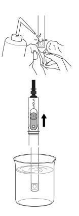
**4. While the pH electrode is immersed in the standard solution, press the** \( \subseteq \) **key.**Stabilization judgment starts and the HOLD icon blinks. When the value is stabilized, the HOLD icon changes from the blinking state to the lit state and the display is fixed to the measured value at the stable time.
