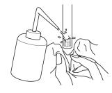
2. Open the internal solution filler port of the ion electrode.
