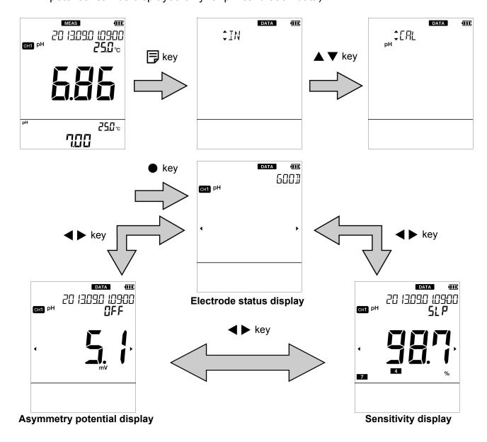
Electrode status based on calibration result
