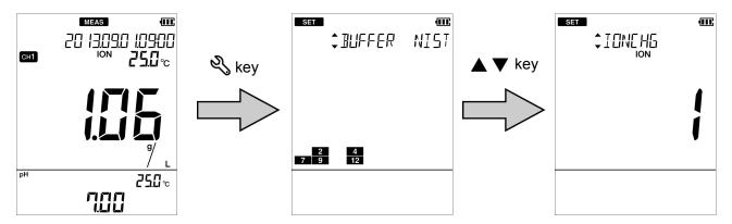
3. Press the ◀▶ keys to select the ion valency and press the ● key.
