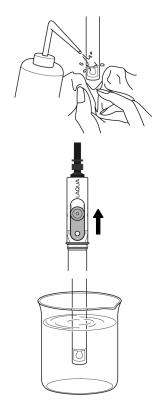
5. While the pH electrode is immersed in the standard solution, press the key. Stabilization judgment starts and the HOLD icon blinks. When the value is stabilized, the HOLD icon changes from the blinking state to the lit state and calibration to the set standard solution value is performed. 1st point calibration ends and the calibration history icon "1" lights, indicating that the 1st point calibration is complete.
