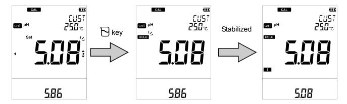
6. Perform the 2nd point calibration. As with the step 2., wash the pH electrode and immerse it in the 2nd standard solution. As with the step 4., immerse at least 3 cm from the tip of the pH electrode.
