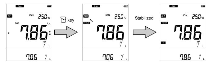
6. Perform the 2nd point calibration. As with the step 2., wash the ion electrode and immerse it in the 2nd standard solution. As with the step 4., immerse at least 3 cm from the tip of the ion electrode.
