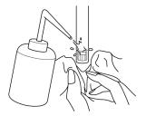
3. Open the internal solution filler port of the ion electrode.
