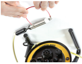
Figure 2 To Test the Entire System: Make sure sensitivity dial is turned fully clockwise. Touch one end of a conductive wire to the probe body and the other end to the probe tip. This will create a short in the probe, the buzzer will sound if the system is okay.
