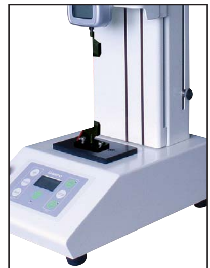
Stand with Optional Grip Performing Tension Test
