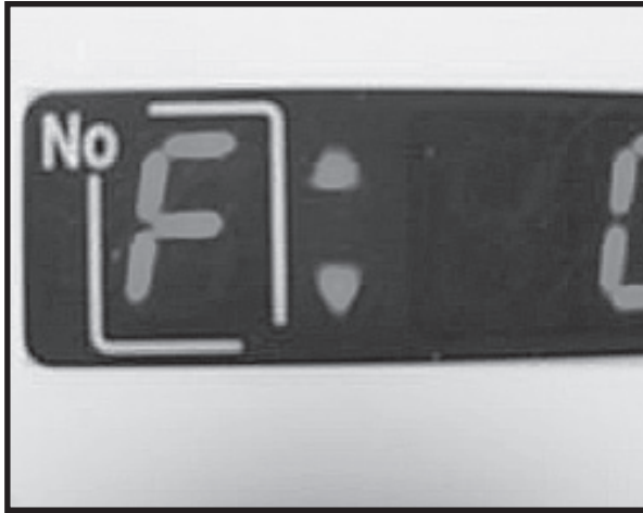
Front panel display indicating force limit for both direction.
