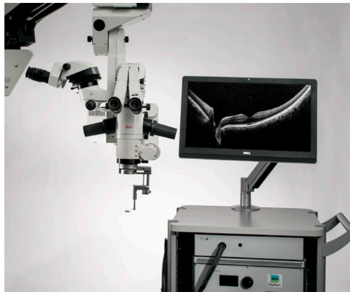
EnFocus OCT can be flexibly shared between different microscopes
