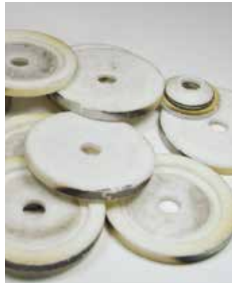
Plastic parts: before and after cleaning with steam and ultrasound
