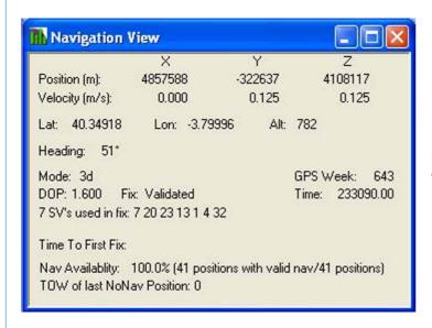
Navigation view, showing the altitude, longitude, latitude, time current parameters and the clock drift.
