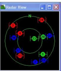
Geographic Azimuth for the positioning of the satellites on the geographic plane together with its identifier, the Azimuth value and the altitude.
