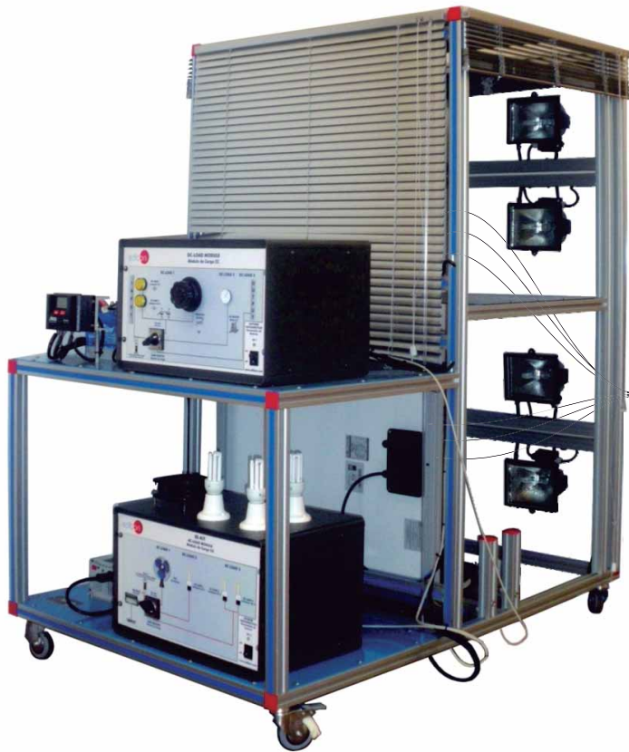
① Unit: EESFC. Photovoltaic Solar Energy Unit
