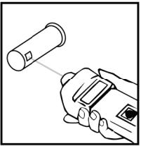
**NOTE:** When switching from the contact to the non-contact mode, the unit RPM will show on the display and also 5 dashes (----). Press the power switch to cancel the dashes.
