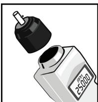
**NOTE:** Hand tightening is sufficient; do not use excessive torque when mounting the DT-ADP-200LR
