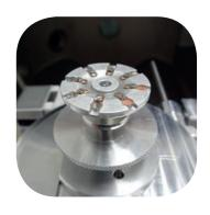
3.05mm TEM specimen grids are easily mounted to the 12 position grid holder. Any combination of bright and dark field diodes (including reversed polarity) may be selected for processing.
