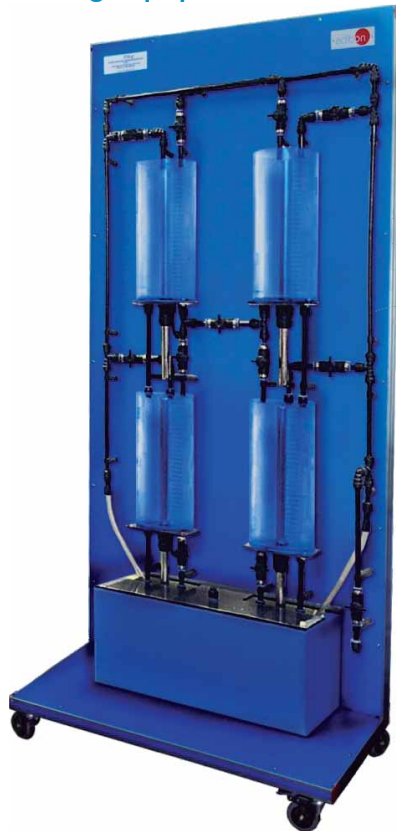
① Unit: CTAC. Coupled Tanks System
