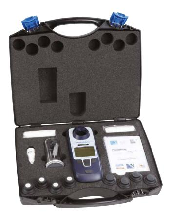
Turbidity and Total Suspended Solids (TSS) are two of the most important indicator parameters for water quality monitoring. The Compact Turbimeter provides the ideal testing platform using unique QuadoptiX™ technology with a sophisticated yet simple to use instrument.
