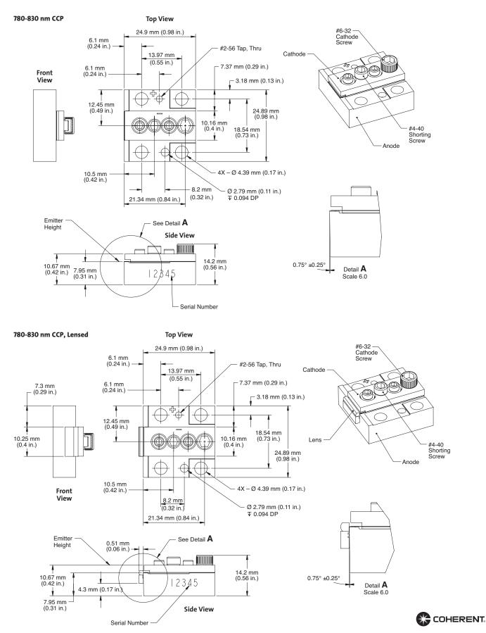
High Power Single-Bar Packages for Pumping and Direct-Diode Applications
