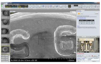
The Deben ballistic bullet comparison stage is a sub-stage designed for use with SEMs and optical microscopes.
