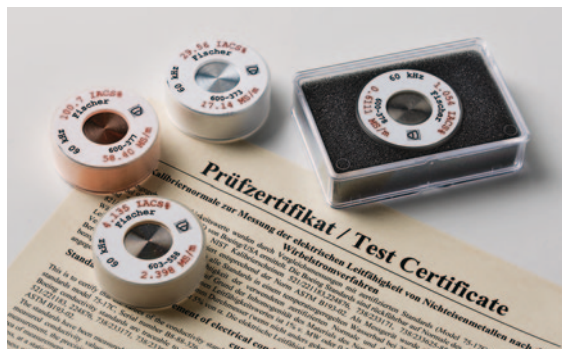
Certified standards for calibrating the SIGMASCOPE® SMP350, traceable to internationally-recognised calibration norms
