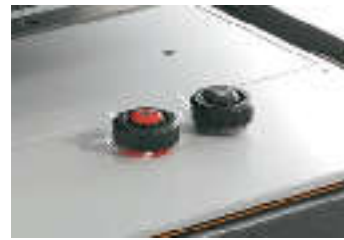
Electrolyte solution measurement cell for the quick and easy analysis of electroplating baths
