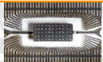
Lead frame: Au/Pd/Ni/CuFe
