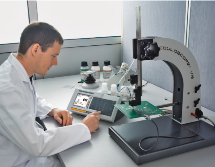
Measuring the thickness of remaining tin on a printed circuit board using the COULOSCOPE CMS2 and support stand V18
