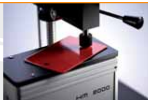
Determining the mechanical characteristics of lacquer coatings
