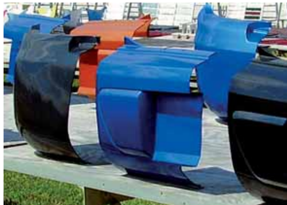
Outdoor weathering site for testing how paint reacts to environmental influences, Picture credit: Atlas Material Testing GmbH
