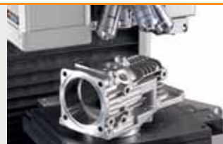
Microhardness determination on a gear housing
